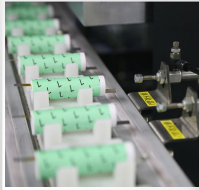
On-line Short-circuit Testing
